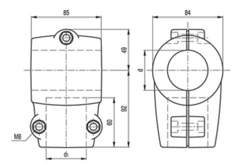
d (inch) = 1 1/2 Gas d1 (inch) = 1 1/2 Gas d1 (mm) = 48.3 d mm = 48.3 Weight (g) = 390
